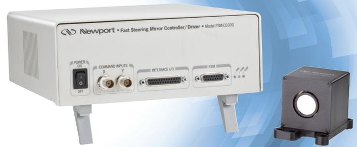
The Fast Steering Mirror Series provides two-axis, high-bandwidth rotation with sub-microradian mechanical resolution using voice-coil technology. Utilizing a unique flexure suspension design to confine the motion of the mirror results in ultra-smooth motion about a gimbal point, very high accuracy, and practically no wear. Newport offers a wide range of 1" field replaceable mirrors.
